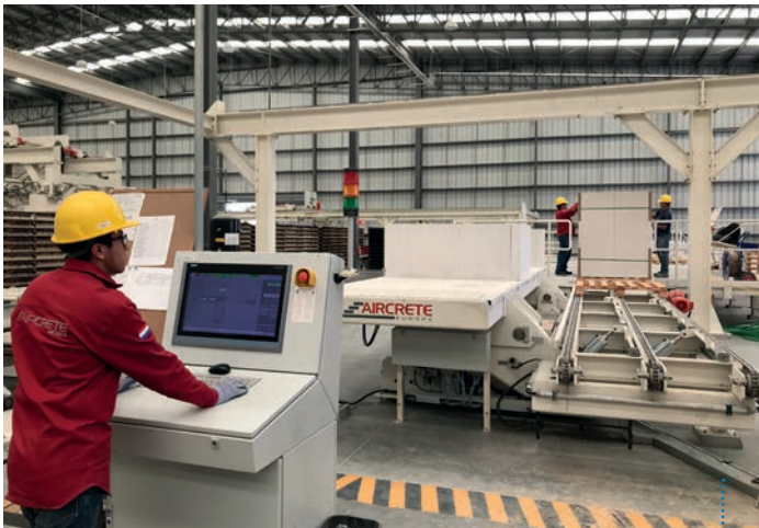
Fig. 4: The control and monitoring modules distributed in various production areas are seamlessly integrated and managed by the overarching in-house developed Aircrete Plant Control System.
