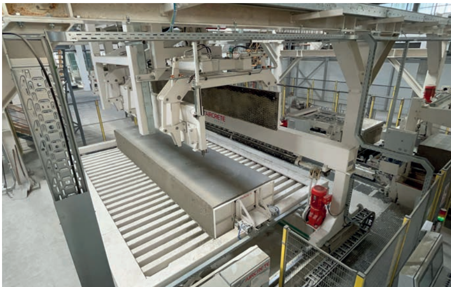
Fig. 6: The view on the Aircrete Separate Cross Cutter (where the lamellas can be seen as well). In the background the green cake (with the cross cut) has been posi- tioned on the next section of the cutting line.
