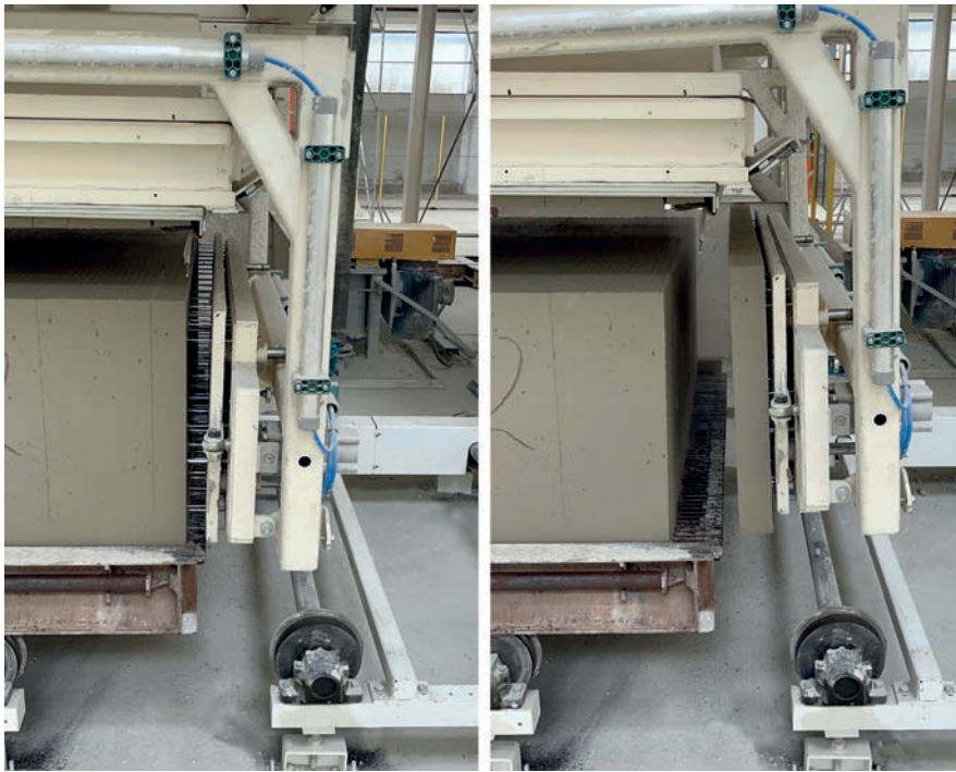
Fig. 7: The side crust being removed by the Needle-plate End-hood Removal System.
