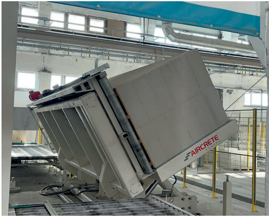
Fig. 8: The tilting table automatically tilts two complete cakes onto six pallets at once.
