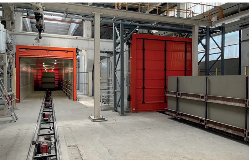
Fig. 9: Newly-installed climate controlled chambers to buffer the green cakes before autoclaving.
