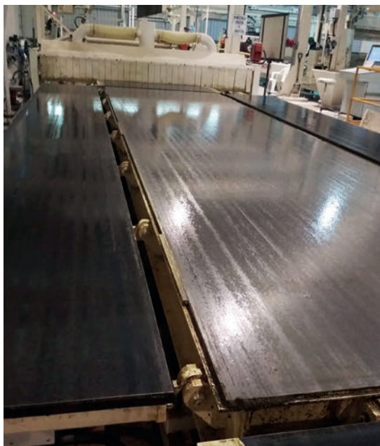
Fig. 5: The Aircrete moulds can be opened completely, which provides a big advantage when it comes to cleaning, which in return prevents quality issues.
