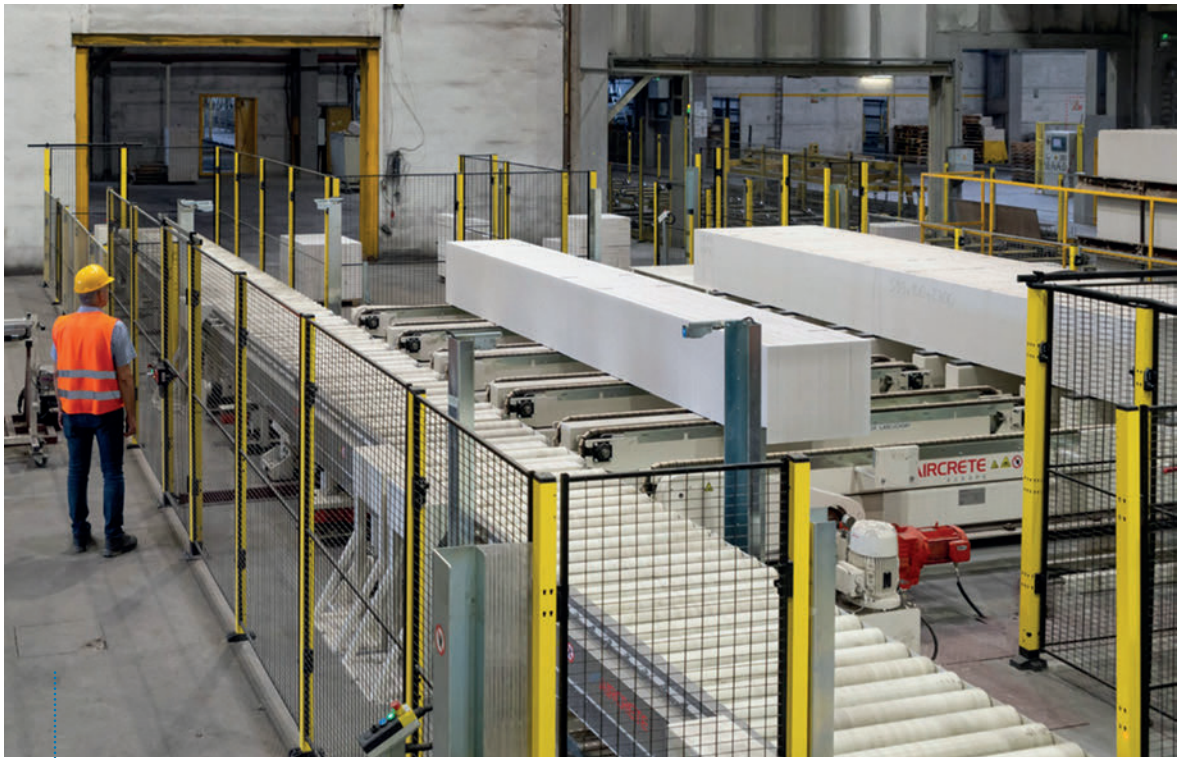
Fig. 9: the Aircrete panel pack configuring system allows for fully automatic configuration of different pack sizes.
